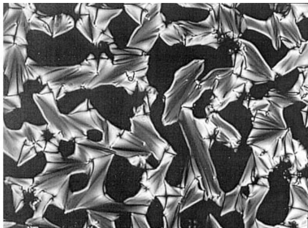
Figure 4. Texture observed for the smectic A mesophase of [\text{La}(\text{dbm})_3\text{L}_2] at 81 °C (clearing point)
